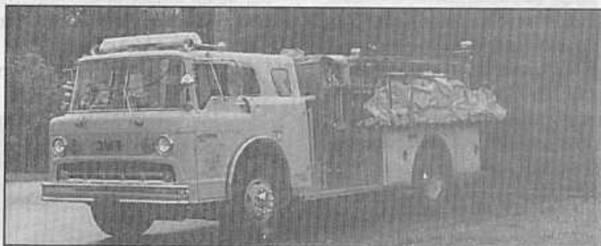
E-322. F.M.C. Firetruck. 1000 Gallon-per minute pumper.
